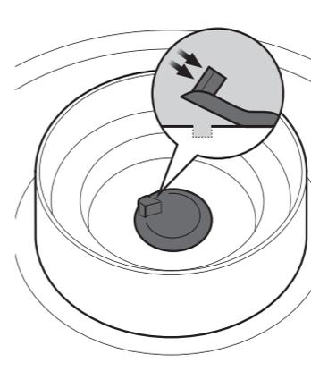
1. After blending, gently lift up one side of the rubber cover to release the pressure.
