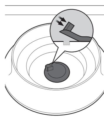
1. After blending, gently lift up one side of the rubber cover to release the pressure.
