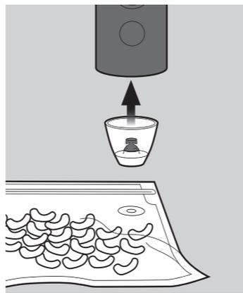
3. Place it on a flat surface and connect the accessory to the pump.
