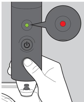
4. Place the pump on top of the air valve. Press the power button once. Wait until the indicator shows all green.
