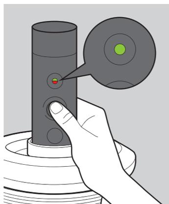
5. Press the power button once. Now the air gets pumped out. The indicator will show all green when finished.
