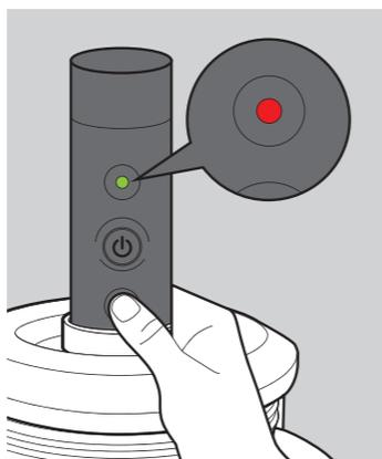
6. Press the pressure release button for a few seconds to release the pressure between the pump and accessory.
