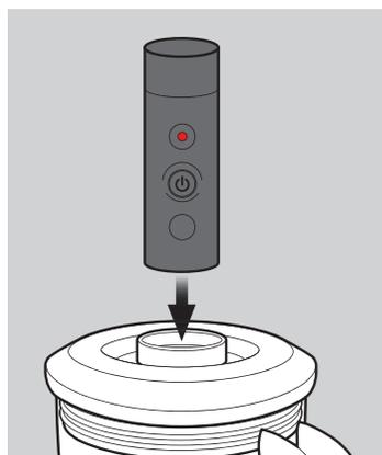
4. Put the vacuum pump onto VPA05.
