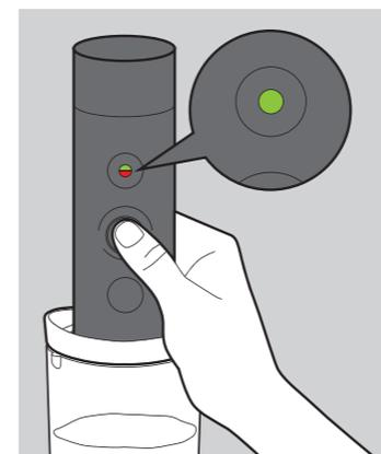
5. Put the vacuum pump onto the lid, then press the power button once. Wait until the indicator shows all green.
