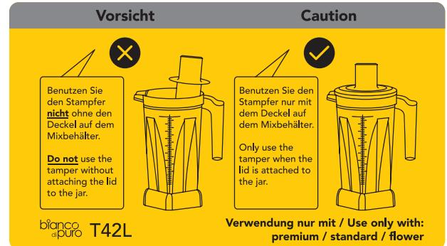
Run the tamper only through the lid opening of the measuring cup. (see Fig. 2, page 1). Use only the provided tamper and **no other** objects to press the mixing content towards the blades. The less water you use, the more you have to work with the tamper. If you use other objects, the device can be damaged.
